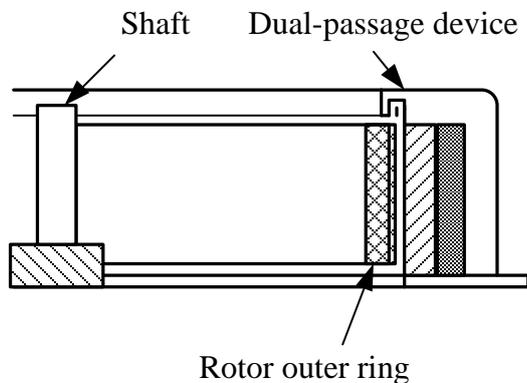
**Figure 12.** Dual-passage device of the computer cooling fan
