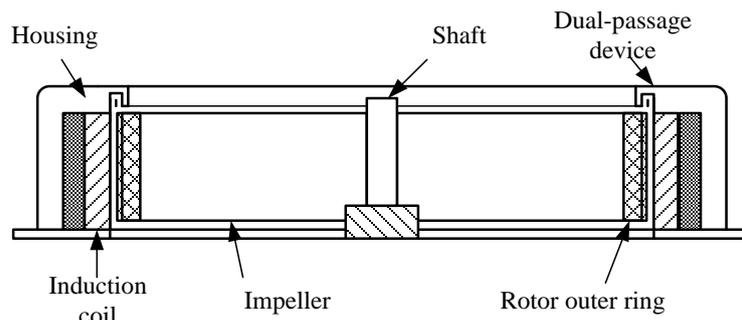
**Figure 11.** New housing design for the computer cooling fan
