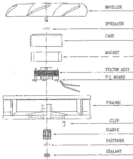
**Figure 3.** Constituent components of a computer cooling fan
