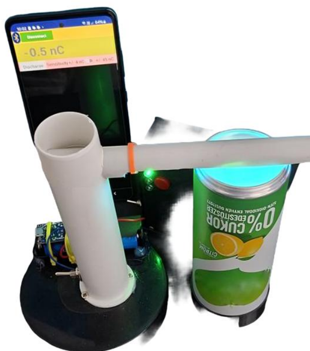
Figure 11. Demonstration of the photoelectric effect (the UV light source is housed in a 3D-printed enclosure to prevent radiation from reaching the surroundings) (Source: Authors' own elaboration)
