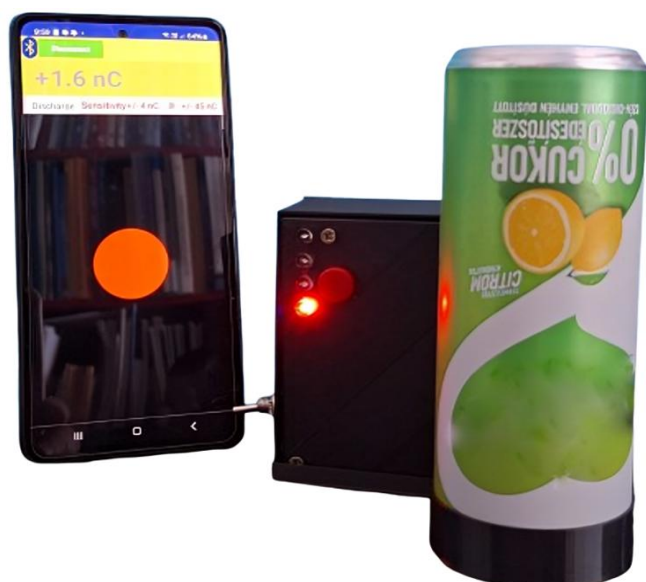
Figure 10. Metal body charged positively by electrical sharing (Source: Authors' own elaboration)
