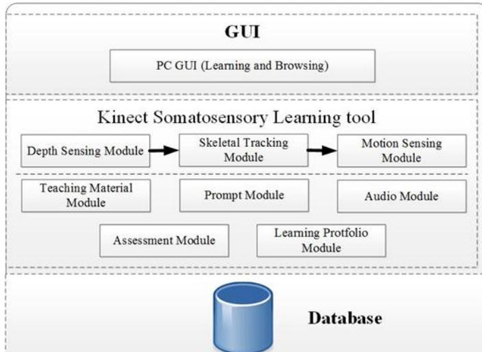
**Figure 2.** System Architecture
