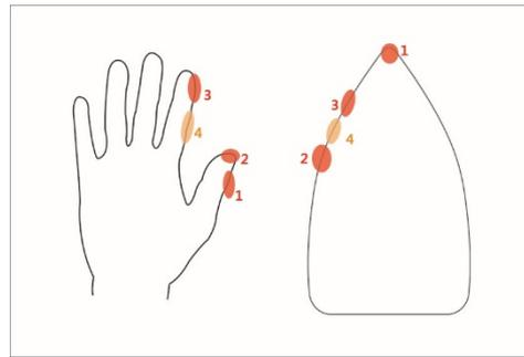
**Figure 6.** Portions of contact between Subject #2's hand and the iron soleplate
