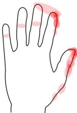
**Figure 13.** Probability distribution for contacts with the iron soleplate on the hand
