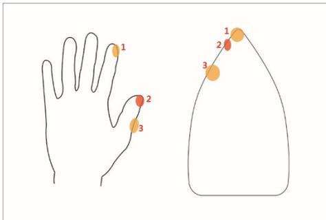
**Figure 7.** Portions of contact between Subject #3's hand and the iron soleplate
