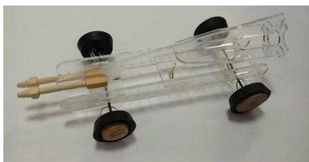
(a) Acrylic laser-cut CO<sub>2</sub> dragsters assembled with additional materials
