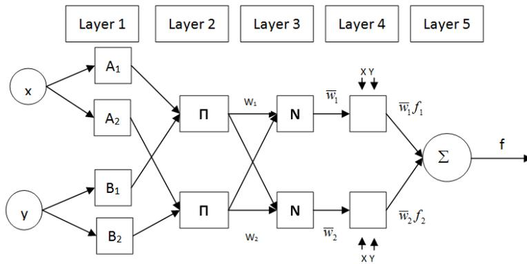
**Figure 8.** The architecture of an ANFIS network
