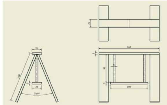
Figure 10. The Material Size Picture of S5
