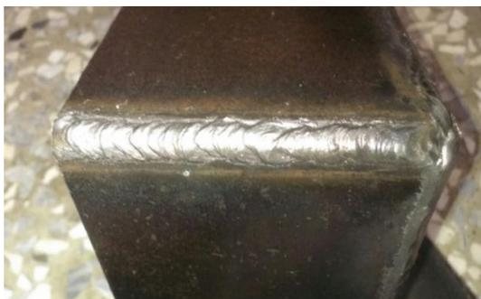
**Figure 19.** Welded Polish and Grinding
