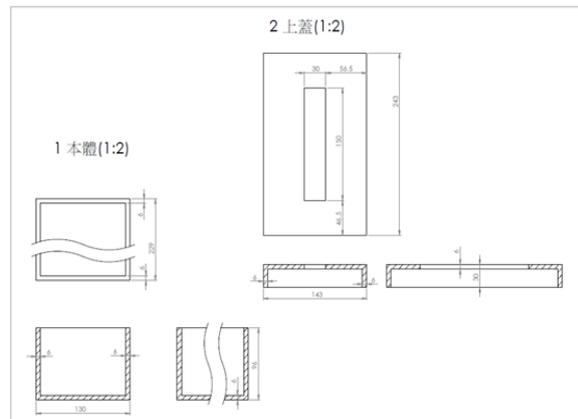
Figure 12. The Material Size Picture of S8
