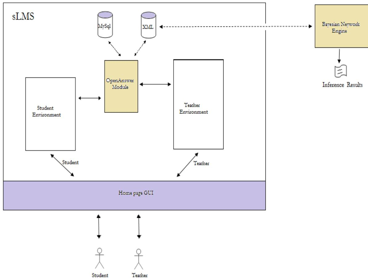
**Figure 3.** The functional architecture of the system: students and teachers can interact, respectively, with the student and the teacher environments through the front-end management modules while the Bayesian Network Module represents the back-end module.
