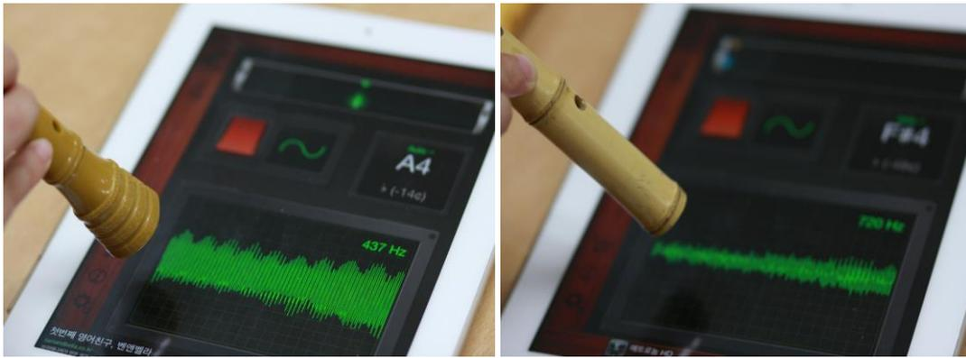
**Figure 3.** Measuring the frequency of a danso with a smartphone application
