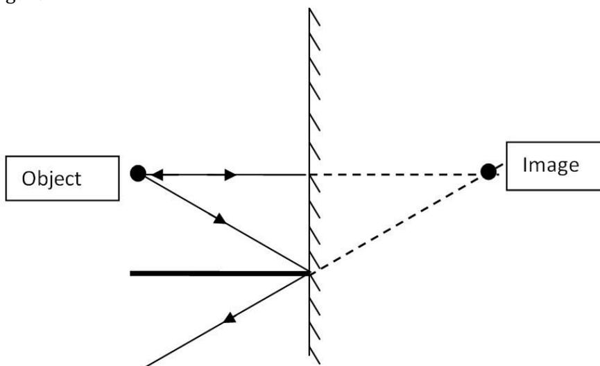
**Figure 1.** Ray diagram for image formation of a point object
