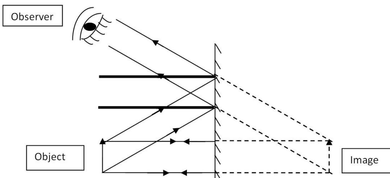
**Figure 3.** Ray diagram for image formation of an extended object
