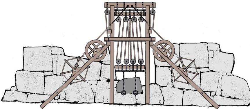
**Figure 6a.** *Geojunggi* was used in the construction of fortress walls
