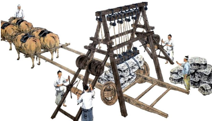
**Figure 6b.** *Geojunggi* was used as a stacker for loading stones
