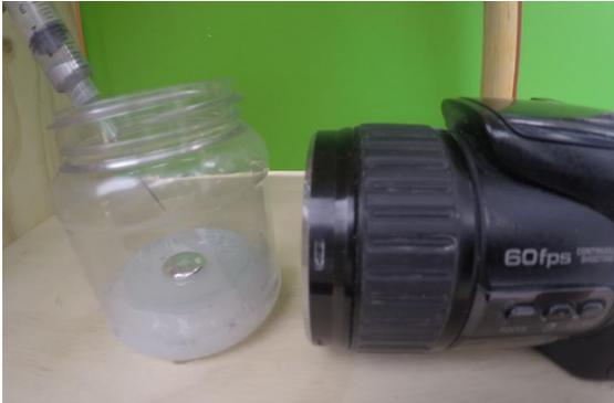
**Figure 7a.** Placing mercury on the glass surface in front of the video camera
