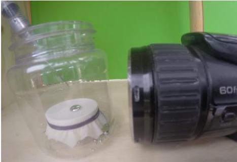
**Figure 9a.** Placing mercury on an elastic surface in front of the video camera
