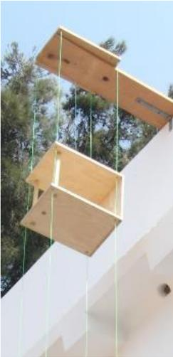
**Figure 6.** Our “elevator” was a semi-open wood box whose fall was guided by four nylon springs
