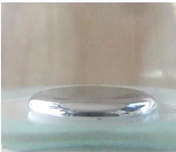
**Figure 7b.** Initial form of the mercury drop on glass surface as “seen” by the camera when the box is at rest
