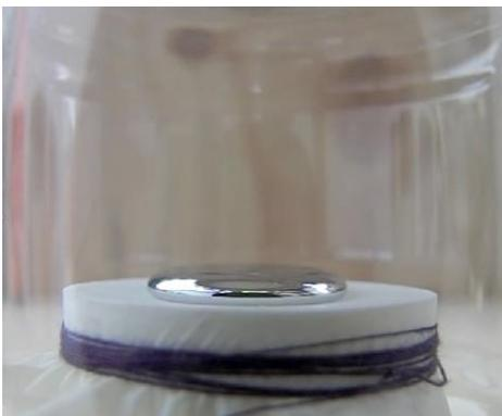
**Figure 9b.** Initial form of the mercury drop on elastic surface as “seen” by the camera when the box is at rest
